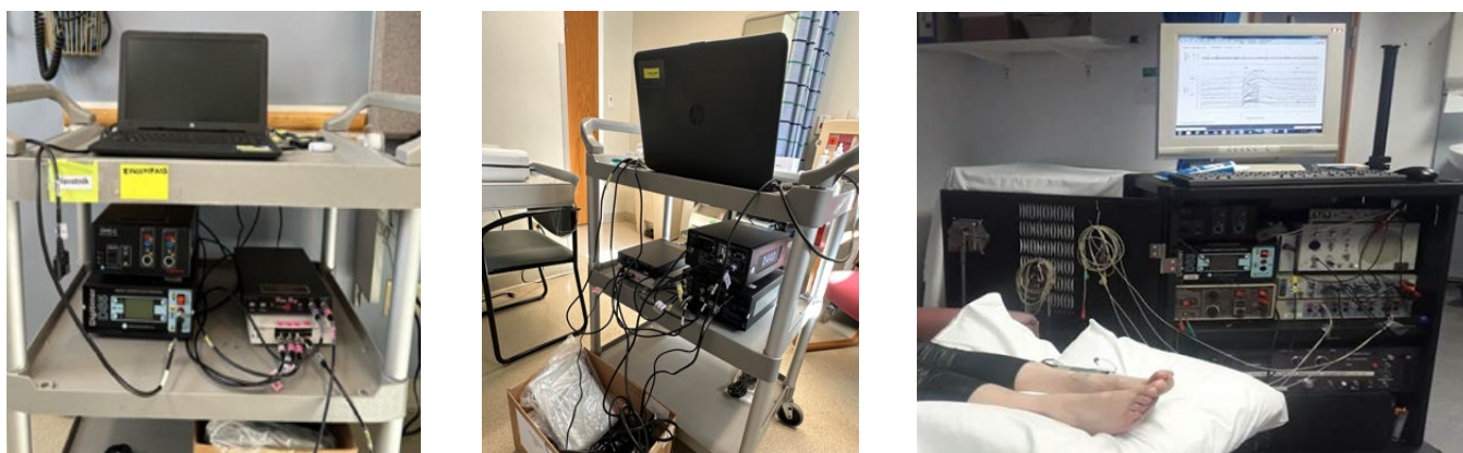
Figure 1. At left is the legacy research system built from off-the-shelf components and developed more than 20 years ago. The standard setup includes multiple cables, a stimulator, a National Instruments analog-to-digital card, an amplifier, and noise-filtering devices. The right image shows a standard microneurography setup including amplifiers and stimulators.
